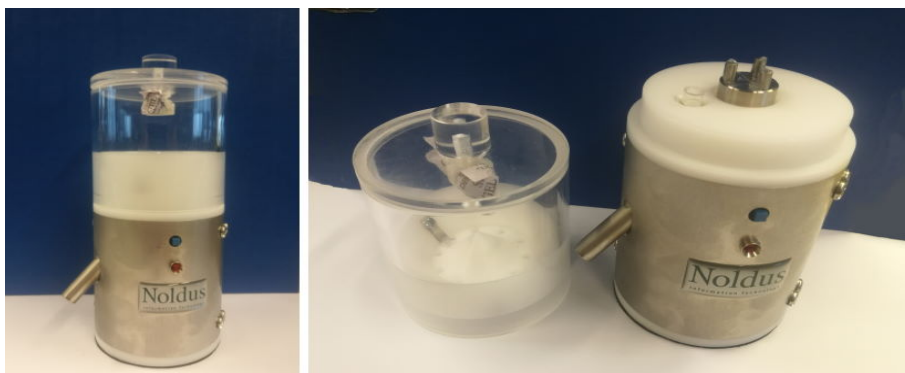
Figure 4.1 Left: Pellet dispenser. Right: The pellet silo and the base part that contains the stepper motor.
