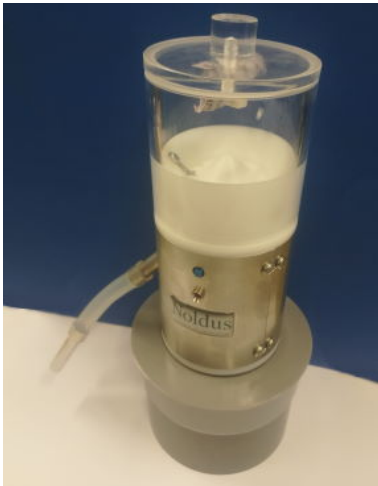
Figure 4.2 Pellet dispenser on its own elevated stand and with aluminium feed-through and silicon in-between tubing.
