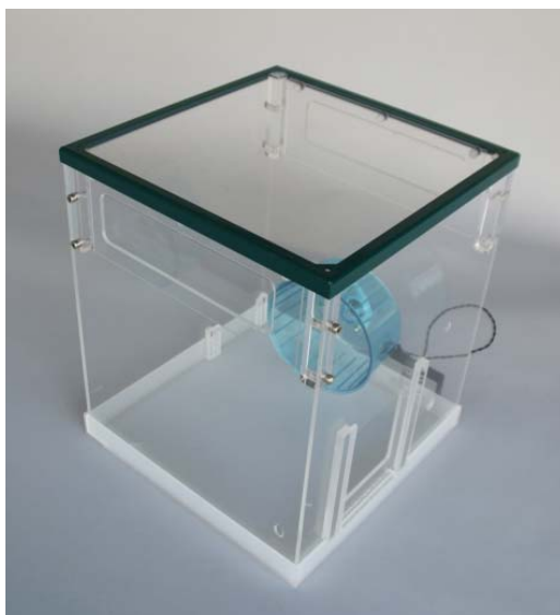
Figure 6.1 PhenoTyper cage with a mounted PTRW-0150 running wheel. On the back side, the counter module.
